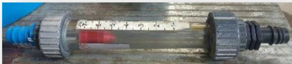
When testing the equipment, the water flow gauge is connected between the sucking pipe and air inlet nipple, before the milk meter inlet. When the vacuum is opened, water starts running through the system and the water flow is read (as shown in picture on the right).
