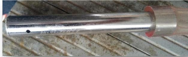
**A nipple with air inlet** 1mm in diameter should provide air intake of  $10 \pm 1$  LPM.
