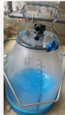
**Suction pipe** with an inlet hole of 3.5mm, which allows a  $4 \pm 1$  LPM (Liter per Minute) flow of water. The entire set should be tested and verified for the defined flow rate (see testing the equipment below). This part will replace the milking claw for the purpose of the test.
