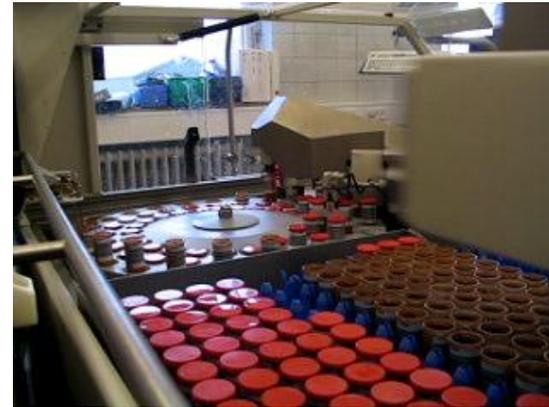
The ILAS robot will identify vials for special analysis, and after the CombiFoss (fat, protein, and cell count ) the racks are moved to the Pic and Place Robot
