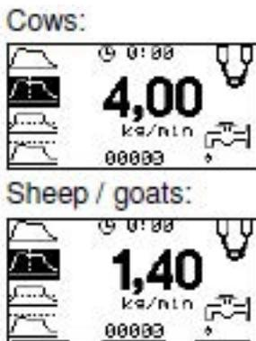
Empty the milk bucket on the floor and ensure that there is enough water in the bucket standing in the cows place to go through this item. Press the start button and the IDCs will suck up water from the bucket. The IDC stops automatically, when desired amount has been sucked and screen image changes to the one displayed in item 3.
