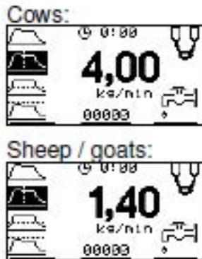
The flow meter is set to suck through the large and the small nozzle at the same time (the flow meter will now suck 4 l/min (cows) or 1.4 l/min (sheep/goats)). Press start and the IDC will suck up water. After about 15 seconds start is pressed again so the IDC stops. This is done to change the amount of water in the IDC, and change the hoses to a high flow.
