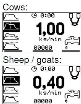
Set flow meter to only suck through the small nozzle (flow meter will now suck 1 l/min (cows) or 0.4 l/min (sheep/goats)). Press "Start" and the IDC start sucking water. Press "Start" again after app. 15 seconds to stop IDC. This is done to alter the amount of water in the IDC and hoses to low flow.
